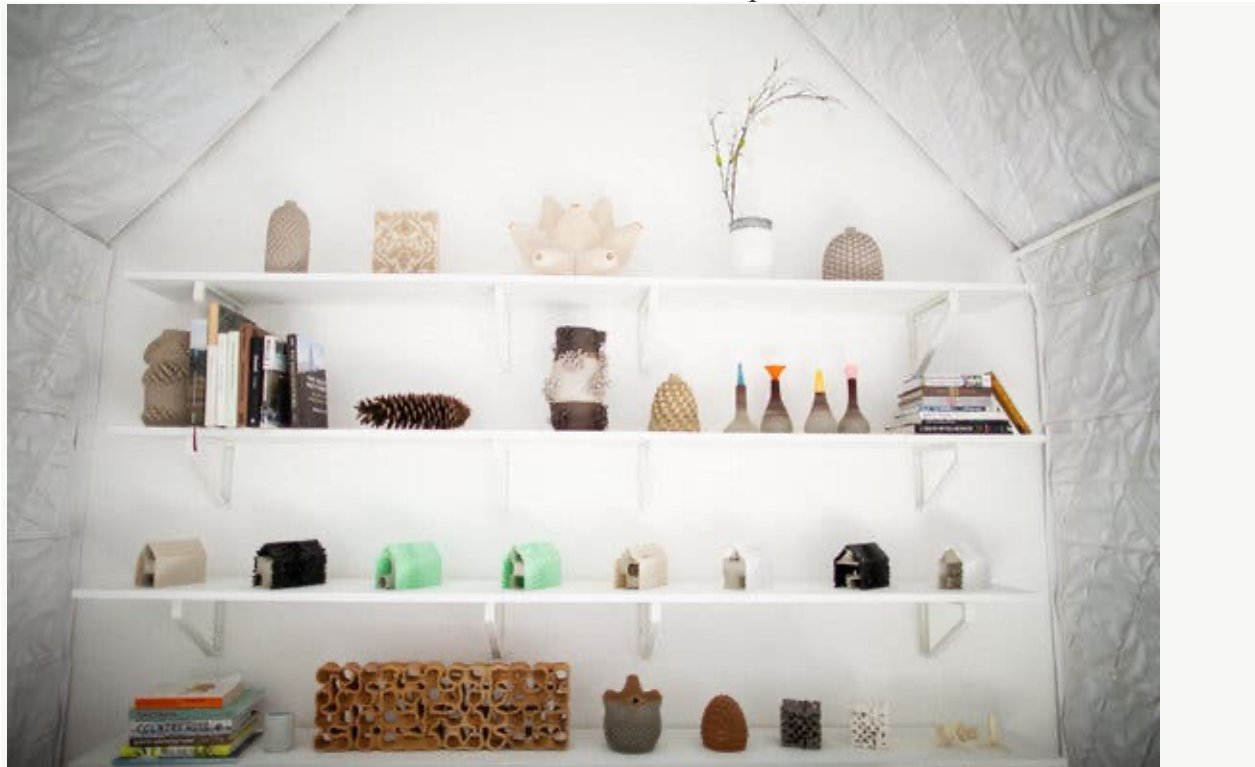
The 3-D-printed vessels, built layer by layer in the process, and 3-D cabin models on the shelves inside the cabin. The walls are composed of layers of bioplastic. Credit... Talia Herman for The New York Times
